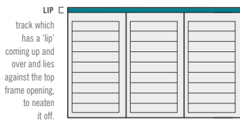
Top track with lip (To neaten uneven walls, window frames, gaps etc)
